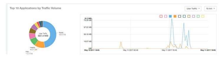
The pie chart and graph contain the top applications with the largest traffic volume in the network, along with the received and transmitted traffic volumes. You can view the received and transmitted traffic volumes based on the Rx+Tx Filter on page 30. To view the top 10 applications, choose from the legend available on the top of the graph. Each application will appear as a separate graph line. If you hover over the line graph a pop-up appears containing the selected details.
