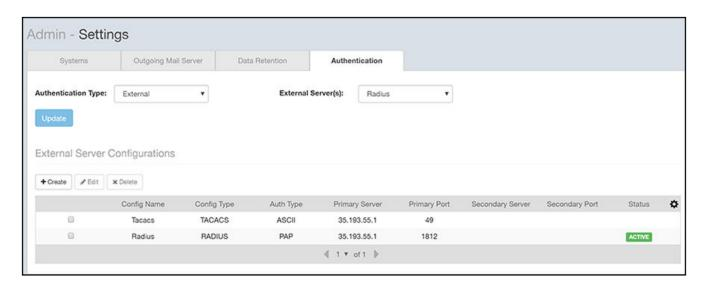
5. (Optional) To edit or delete an external server, check the box for the server, then use the **Edit** or **Delete** buttons as desired.
