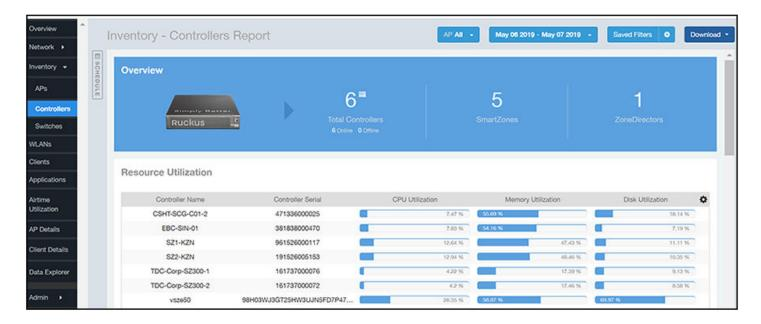
The Inventory - Controllers Report consists of four sections, which are listed in the table below. Figures showing each of these sections appear later.
