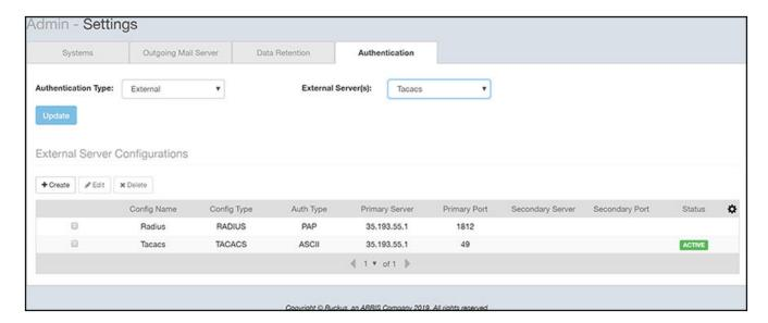
2. Click the External Server(s) drop-down list to view all configured external servers. The figure below shows such an example:
