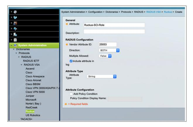
5. Install a new Ruckus dictionary file or update an existing dictionary with the following attributes to create the Ruckus-SCI-Resource-Group (see figure below):
