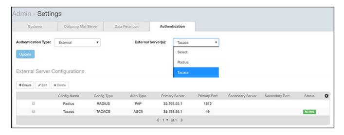
3. From this drop-down list, select the external server from which users must be authenticated. You can select only one such server. If a user is not associated with that server, that user cannot be authenticated and will not be able to log in to SCI.
