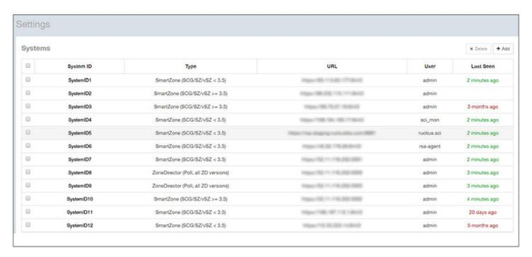
To add a controller, click the **Add** button in the upper right of the Settings screen; a drop-down menu appears for you to select the controller type, as shown in the figure below.
