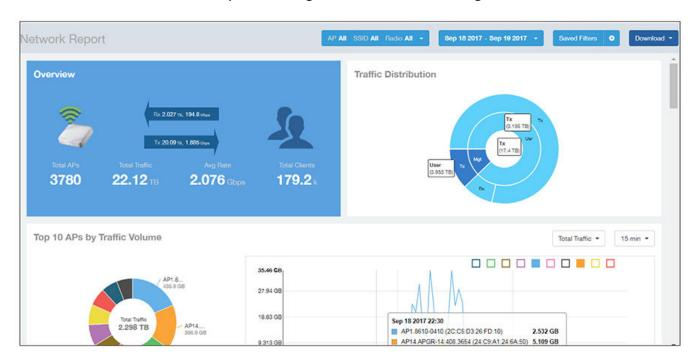
2. Make the desired selections to any filter. In the example figure below, no changes are made to the Radio or Date filters, but in the Top 10 APs by Traffic Volume filters, the Traffic and time-increment drop-downs have been changed to Rx Total and 1 day, respectively.
