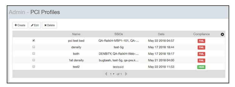
This screen lists the names of the various reports that have been run, the SSIDs on which each report has been run, the date of each report, and whether the overall report passed or failed the PCI compliance test. You can click on the red "Fail" or green "Pass" to observe the detailed report.
